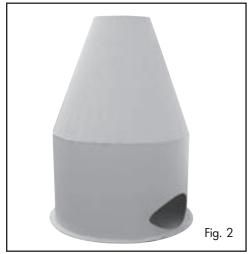
**TECH TIP:** Cyclones are an important part of the filtration process. Damage, excessive wear, holes or corrosion will disrupt the efficiency of the cyclone separator. If any of these issues exist, replace the cyclone immediately. Use a silicone caulk to seal between the mounting lip provided on the cyclone to the support plate in the cyclone chamber in the body.
