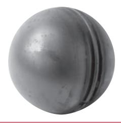
**TECH TIP:** When float balls become worn from years of service, they often fill with material and no longer float. This may cause the unit to carry liquids over into the baghouse and cyclone — resulting in over filling the unit. Check float balls monthly for any signs of wear or damage to ensure proper operation.
