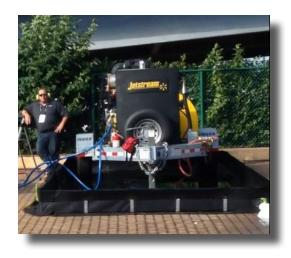
Spill containment and access water run-off from your truck or waterblaster can be a major concern for many.
